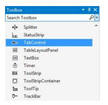
These controls include FlowLayoutPanel, TableLayoutPanel, GroupBox, Panel, TabControl, and SplitContainer.
