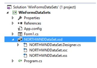
6. Click the dataset node in **Solution Explorer** to open the dataset in the **DataSet Designer**. Each table in the dataset has an associated TableAdapter object, which is represented at the bottom. The table adapter is used to populate the dataset and optionally to send commands to the database.
