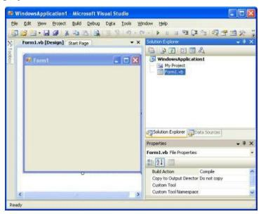
ix) The Properties Window: The properties window is divided into two columns of text, with the properties on the left, and their setting on the right. The object you're setting properties for appears in the drop-down list box at the top of the Properties Window, and you can select from all the available objects using that list box.
