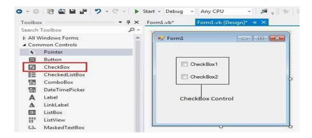
The CheckBox control has three states, **checked**, **unchecked** and **indeterminate**. In the indeterminate state, the check box is grayed out. To enable the indeterminate state, the *ThreeState* property of the check box is set to be **True**.
