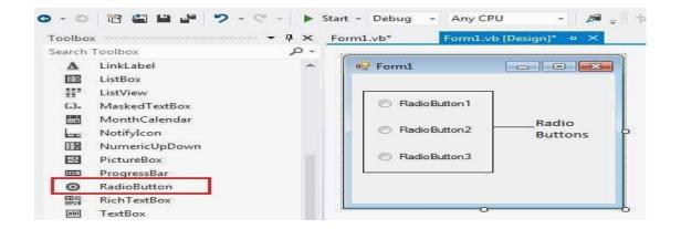
The *Checked* property of the radio button is used to set the state of a radio button. You can display text, image or both on radio button control. You can also change the appearance of the radio button control by using the *Appearance* property.
