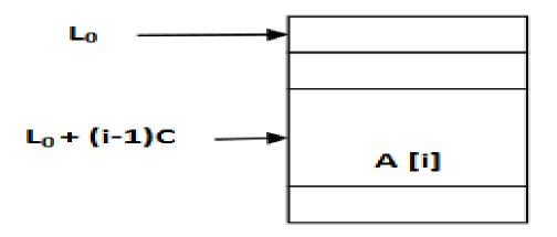
L0- the address of the first word allocated to the first element of vector A.
